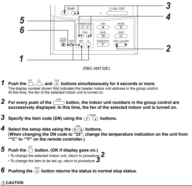
Be sure to perform the item code (DN) set up as "Cooling Only" for the cooling only indoor unit in case of a heat recovery type. If this setting is not performed, error code [L18] may occur.
