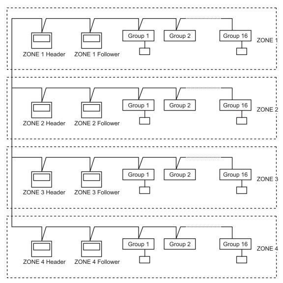
\* In case of "1:1 model" (Super digital inverter / digital inverter), follower indoor units in a group control and twin control must not be counted as "one unit". In the case of VRF system, follower indoor units in a group control must be counted as "one unit".
