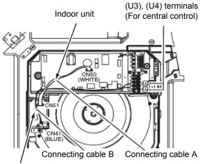
U3, U4 1:1 model terminal connection Indoor block for Relay interface board control PCB connection wire (A) Spacer (A) A CN050 (White) 000 0
