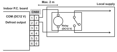
ON signal output when outdoor unit is in "defrosting" (when receiving defrost signal from outdoor unit)
