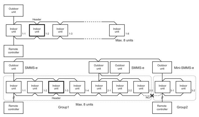
In case of DI/SDI, each Header indoor unit connected with outdoor unit controls room temperature according to setting on the remote controller. The Header indoor unit in the group is the representative of multiple indoor units and sends/receives signals to/from the remote controller and other indoor units in the group.
