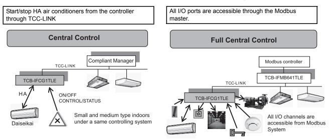
The actions of air conditioners and relay output control corresponding to changes of status at input ports are programmable on site. Relay outputs can form logic circuits. (Control Pattern Programming: combination of 2 analog and 5 digital inputs in 12 patterns)
