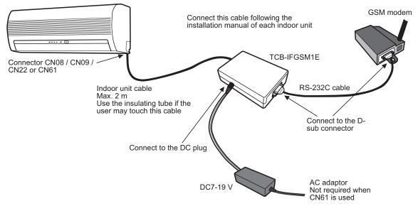
The cable connected to the CN61 and CN4 should be the optional connector cable TCB-KBCN61HAE.
