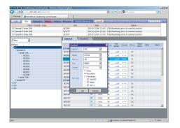
Settings can be easily changed by floor / tenant / area in a batch or by each air-conditioner
