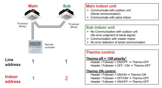
(Note) When remote controller sensor is selected, both indoor units use remote controller sensor as "TA sensor".
