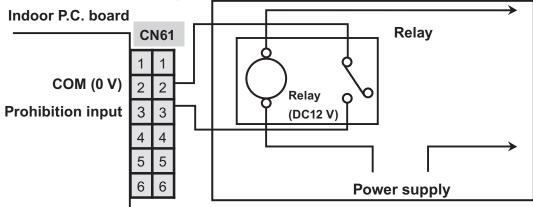
When signal ON, Remote controller ON/ OFF is prohibited. Central controller becomes Central 1 (ON/OFF Prohibited) mode.
