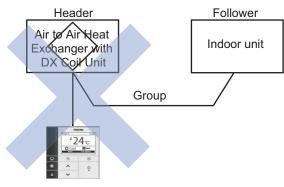
·Ventilation unit is set to header of group operation
