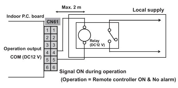
(Note) Individual signal output group control is available. If follower indoor unit generates alarm, signal becomes OFF in this indoor unit only.
