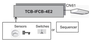
By using TCB-IFCG1TLE, you can program actions of indoor units and relay output corresponding to changes of status at input ports on site as well as the controller can access devices connected to I/O ports through the TCC-Link.
