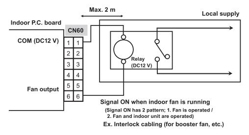
(Note) Signal is OFF when 4-way cassette type performs intermittent operation after oil recovery control.
