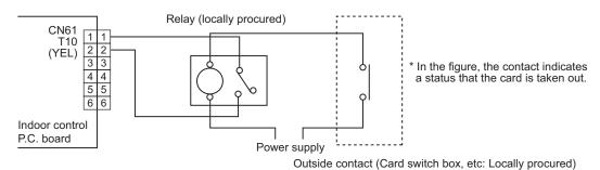
Note) Determine the cable length between the indoor control P.C. board and the relay so that they are within 2 m.
