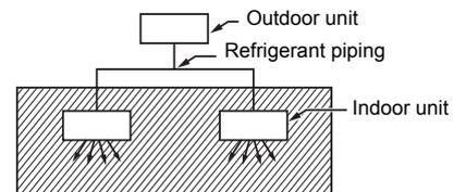
(3) If an indoor unit is installed in each partitioned room and the refrigerant piping is interconnected, the smallest room of course becomes the object. But when a mechanical ventilation is installed interlocked with a gas leakage detector in the smallest room where the density limit is exceeded, the volume of the next smallest room becomes the object.
